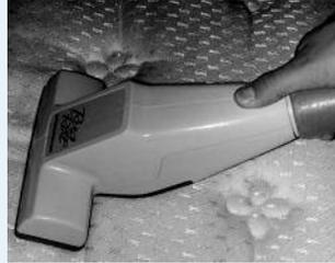
Some companies report that a separate HEPA-filtration vacuum cleaner makes a more positive impression than vacuum tools attached to extractors or truck mounts. In addition, it is recommended that technicians wear dust masks or respirators during vacuuming. This is for their protection as well as to make a value added impression on the customer.
